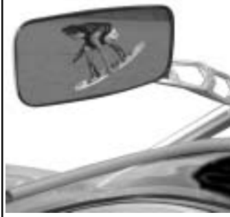
Tower Mounted Mirror
