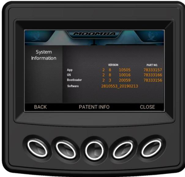
The System Information screen provides the version and part number for the Application, Operating System, Bootloader and Software. This information will be useful should the unit require troubleshooting.
