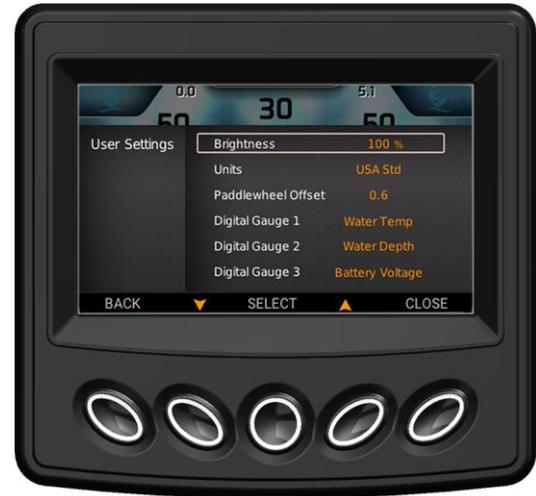
Paddlewheel Offset and press Select. The arrow keys then become – and + to adjust the offset. Press the button below Done when finished.
