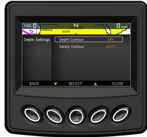
Set the Safety Contour value to a water depth above what the vessel can safely navigate:
