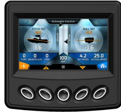
Once the button is pressed to turn on AutoWake, the system will try to first fill to establish the correct roll, then it will fill all the rear ballast until rear “Amplitude” is achieved. It does this in Static mode when the boat is traveling less than 3 mph and in Dynamic mode when the speed is within .1 of set speed. If AutoWake is active, achieved or in countdown, it will
