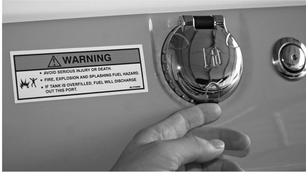
The fuel cap is located on the rear deck, 2-4 feet from the stern. To open, push black tab located on the bottom side of the gas cap. When the black tab is pushed, the gas cap will hinge upward.
