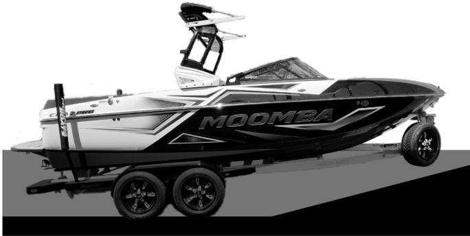
**NOTE: DO NOT attempt to use excessive power to free the boat from dry carpet runners. Power off of the trailer only when the boat has floated free.**
