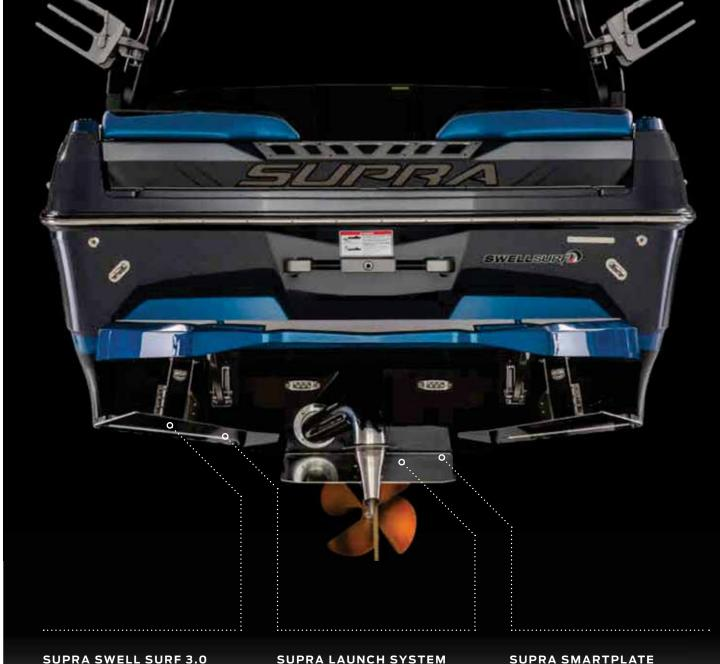
We optimized the Supra Swell™ Surf System to provide tall waves with long pockets and optimal push that's consistent on both sides of the wake—the perfect waveshaping tool for riders who love to transfer from side to side.
