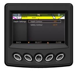
Set the Safety Contour value to a water depth above what the vessel can safely navigate:
