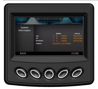
The System Information screen provides the version and part number for the Application, Operating System, Bootloader and Software. This information will be useful should the unit require troubleshooting.
