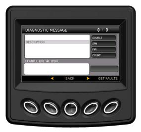
The Diagnostic Message area will provide a description of an existing fault and a corrective action, if necessary. Also present will be the source, SPN, FMI and count information
