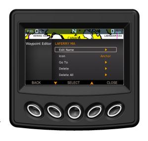
Selecting Delete All will display a pop-up screen to confirm the deletion of all waypoints. Press the appropriate display key under the desired action to perform.
