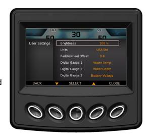
Paddlewheel Offset and press Select. The arrow keys then become – and + to adjust the offset. Press the button below Done when finished.
