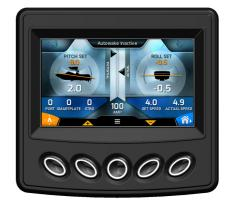
return to inactive if a ballast switch is used, speed is not between 7 mph and 26 mph, or cruise set speed is not within 7 mph and 26 mph. If the display is powered down, it will come back with AutoWake off.
