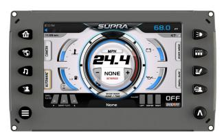
The cruise control can be turned ON or OFF from this screen by touching **[ZEROOFF]** located in the lower right of the screen.
