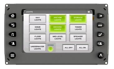
**NOTE**: If the cell is gray, this indicates the lights are OFF. If the cell is green, this indicates the lights are ON.
