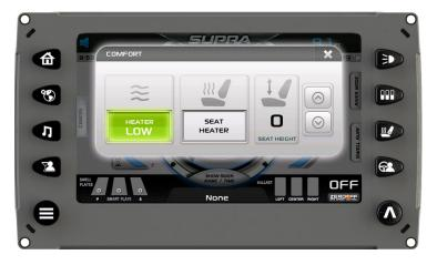
**NOTE**: If the cell is gray, this indicates the settings are OFF. If the cell is green, this indicates the settings are ON.
