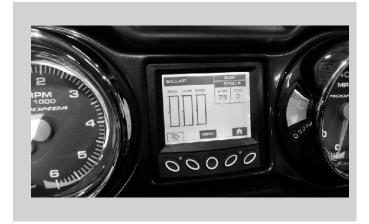
The Ballast System in your boat is electronically controlled and can be operated from the driver's seat. The manual switches for this three position system can be located ito the right of the steering wheel.
