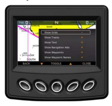
To show or hide grids, tracks, text, navigation aids, waypoints or waypoint names, highlight the desired setting and press TOGGLE. The asterisk will illuminate (show) or dim (hide).
