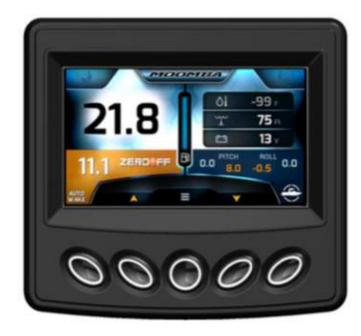
When AutoWake is active, the Ballast levels normally shown on the right side of the screen will be replaced with the Pitch and Roll values.
