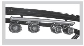
The tower lights are designed to make docking, loading and unloading easier. The tower lights require the addition of a dual-battery electrical system.
