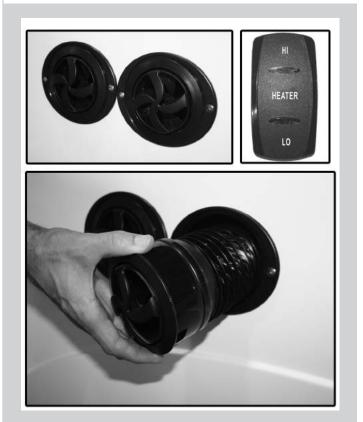
The boat heater is a forced air heater that uses hot engine water as a heat source. To use the heater, simply turn the heater switch to the selected fan speed. In order for the heater to work, the engine must be at operating temperature. One of the features of the heater are the snorkel vents, which can be pulled out to direct heat to specific areas.
