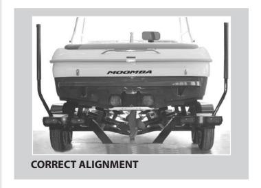
When pulling the boat onto the trailer, be sure that it is centered on the trailer.
