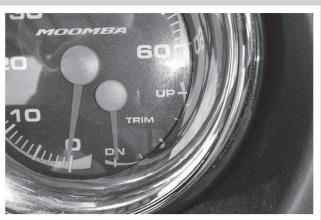
The Wakeplate switch controls the position of the center trim tab (wakeplate). The corresponding trim guage dictates the position of the wakeplate. The down position raises the stern of the boat and lowers the bow. The wakeplate helps shape the wake for surfing and wakeboarding.
