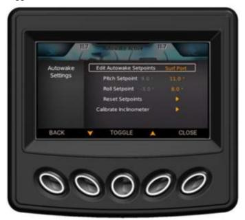
**Edit AutoWake Set Points:** Use the arrow keys to highlight this selection and press the Toggle button to choose Surf Starboard, Surf Port or Wake.
