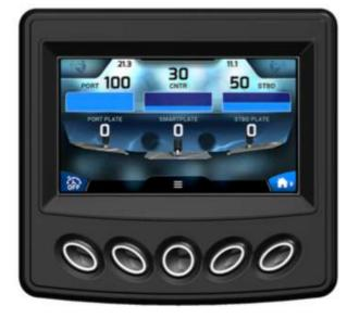
This screen retrieves information from the PDM regarding the amount of fluid in each ballast, along with the position of the Port and Starboard plates and the Smartplate.
