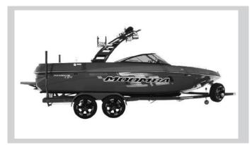
The trailer supplied with your Moomba model was designed especially for the boat with your convenience in mind. Please be sure that you have an appropriate tow vehicle before attempting to trailer your boat. Your vehicle must be capable of towing 4,500 — 6,000 lbs., depending on the model.
