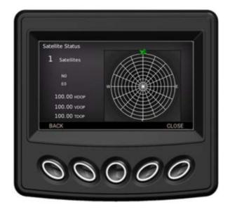
The Satellite Status screen displays the detectable satellites in the area of the craft. Press the display key under Back to return to the previous screen or Close to return to the main screen.
