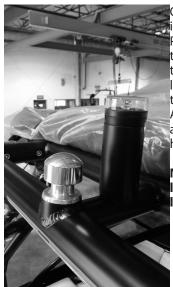
On boats equipped with factory installed towers, the 360° White Pole Light is mounted on the tower. To raise the light, pull the lever on the side of the light and then carefully raise the light to a vertical position. Always lower the light after use and before trailering to avoid hitting low overhangs.
