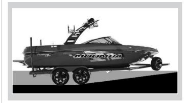
NOTE: DO NOT attempt to use excessive power to free the boat from dry carpet runners. Power off of the trailer only when the boat has floated free.
