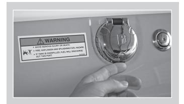
The fuel cap is located on the rear deck, 2-4 feet from the stern. To open, push black tab located on the bottom side of the gas cap. When the black tab is pushed, the gas cap will hinge upward.
