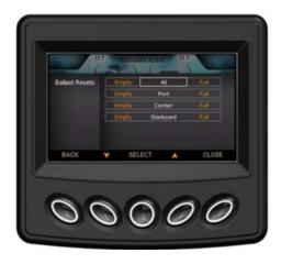
Use the arrow keys to highlight All, Port, Center or Starboard and press Select. Utilize the - (Minus) key to include Empty in the highlighting (shown below around Port) or the + (Plus) key to include Full in the highlighting. Press the display key under Done when finished.
