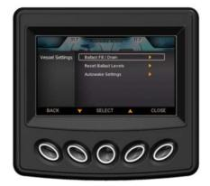
Ballast Fill / Drain: Use the arrow keys to highlight Ballast Fill / Drain and press Select.
