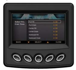
Highlight the particular ballast to be filled or drained and press Select. Utilize the + and - keys to adjust the fill/drain times, then press the display key under Done.
