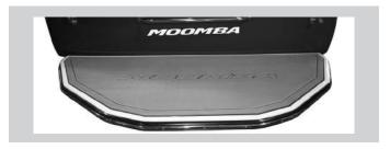
All Moomba models are equipped with a ski platform on the stern. The platform allows easy access to and from the water for skiers and swimmers. It is recommended that all entries to and exits from the water be made from the platform to avoid accidents. (The fiberglass deck can become slippery when wet.)
