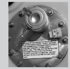
Your boat contains a fuel system that is designed using current fuel delivery technology. The common terminology for this type of system is: Pump in Tank.
