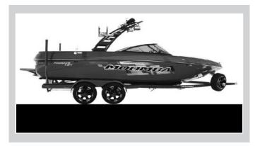
To re-trailer the boat, position the trailer in the water with approximately 1 inch of the top of the fender showing as in step 3. UNLOADING.
