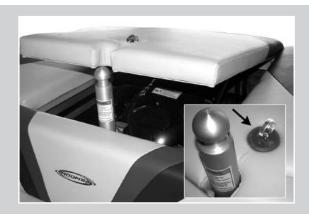
To access the engine compartment, turn latch and pull to raise the center sun deck lid. When the ski lockers and engine compartment lids are closed, the upholstered lids double as a cushioned sun deck.
