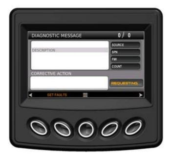
The Diagnostic Message area will provide a description of an existing fault and provide a corrective action, if necessary. Also present will be the source, SPN, FMI and count information.
