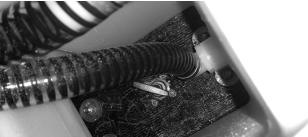
On V-drive models the center drain plug is accessed via the access cover in the center floor panel.
