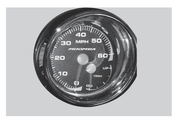
The speedometer indicates the water speed of the boat in miles per hour. It is recommended that the speedometer be checked for accuracy after each 100 engine hours.
