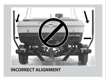
The distance between the boat and the wheel runner board should be about equal on both sides.
