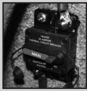
The power to the dash circuit is protected by a circuit breaker that is located in the observer seat storage area near the battery.
