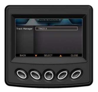
Highlight the desired track and press the display key under Select. The following Track Editor screen will appear:
