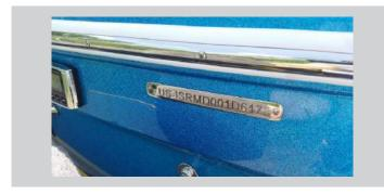
The hull identification number is located on the upper right hand side of the transom below the rub rail.
