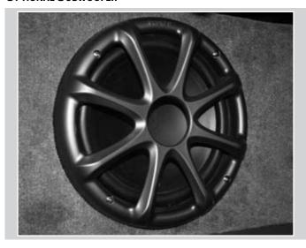
The optional sub-woofer is designed to increase the sound level of the bass notes. The optional amplifier powers the sub-woofer. The bass level can be adjusted on the amplifier. Please see stereo amplifier owner's manual for more information.
