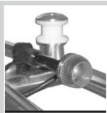
installed towers, the 360° White Pole Light is mounted on the tower. To raise the light, pull the lever on the side of the light and then carefully raise the light to a vertical position. Always lower the light after use and before trailering to avoid hitting low overhangs.
