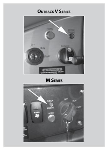
Your boat has an red check engine light. It functions much the same as the check engine light in your car. If the engine control module senses certain engine parameters out of range or a trouble code is set, the light will come on.
