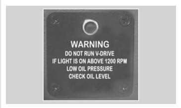
The warning light should be "on" at idle. If the light remains "on" when the engine is above 1200 RPM, shut the engine off and check V-Drive oil level.
