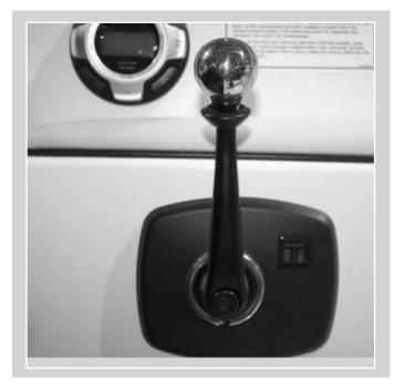
The throttle lever controls both the throttle and the transmission. The idle position (normally vertical) is the zero throttle position and the neutral position for the transmission. A safety ring (umbrella) keeps the lever from being accidentally moved to engage the transmission.
