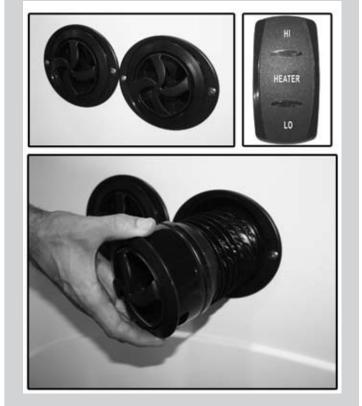
The boat heater is a forced air heater that uses hot engine water as a heat source. To use the heater, simply turn the heater switch to the selected fan speed. In order for the heater to work, the engine must be at operating temperature. One of the features of the heater are the snorkel vents, which can be pulled out to direct heat to specific areas.
