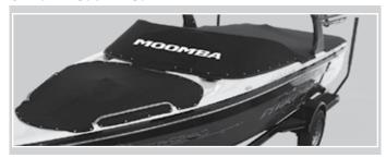
The optional cockpit cover is a snap down storage cover designed to help protect the interior of your boat. To install the cover, start at the windshield and work towards the transom. Be sure to install the cover poles to prevent water pocketing.
