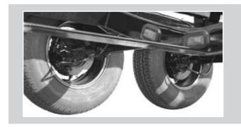
The standard second axle disk brakes give the trailer more stopping power.
