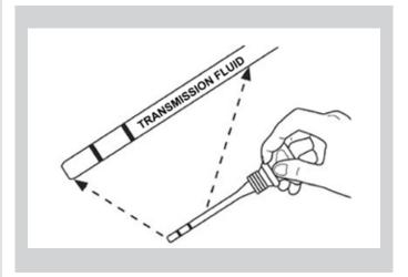
Use only Dextron III transmission fluid in transmissions with 1:1 drive train. To check fluid level, refer to Engine Manual.
