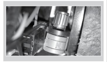
Speed may be checked using a stopwatch and a standard slalom course. Adjust the speedometer needle by twisting the adjuster knobs located beneath the dash panel.
