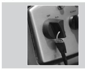
Two ignition keys are provided with the boat. Key entry into the ignition may sometimes be difficult due to the rubber boot protector. Please do not unduly force the key into the ignition. Key tumblers are located vertically, so the key should be vertical when placed into the switch.
