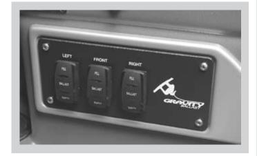
The Gravity Ballast System in your boat is an electronically controlled ballast system that can be operated from the driver's seat. The manual switches for this three position system are located in the switch panel directly below the shifter mechanism.
