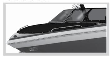
The optional tonneau cover is designed to snap over the bow of the boat. Its purpose is to minimize air flow into the cockpit area when the boat is in use and as a storage cover when used in combination with the optional cockpit cover.
