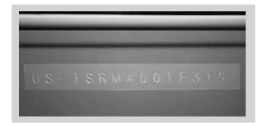
The hull identification number is located on the upper right hand side of the transom below the rub rail.
