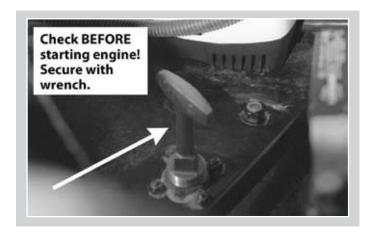
The bilge area drain plug is located at the front of the motor well, in the center under the engine.
