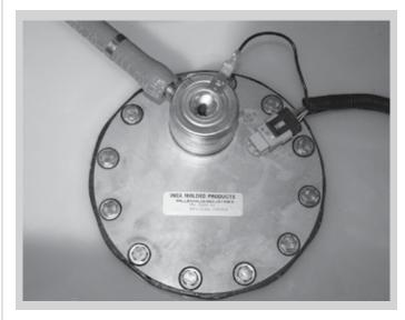
Your boat contains a fuel system that is designed using current fuel delivery technology. The common terminology for this type of system is: Pump in Tank.
