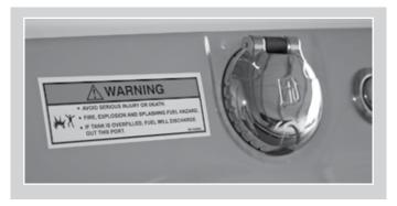
The fuel cap is located on the rear deck, 2-4 feet from the stern. To open, push the black tab located on the bottom side of thegas cap. When the black tab is pushed, the gas cap will hinge upward. To close, push the gas cap down. When the gas cap is completely closed a "click" sound should be heard. The audible "click" ensures that the gas cap is closed and sealed.
