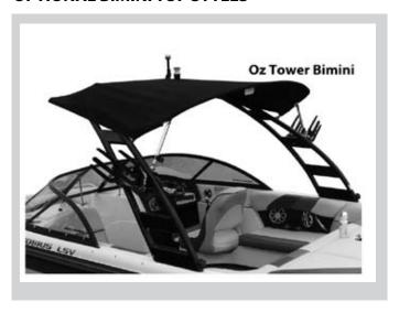
The bimini top is designed as a sunshade. Please see the mooring cover section for instructions on cleaning and caring for your bimini top. When opening and latching the straps to the eye hooks, twist the strap one to two times to prevent them from vibrating in the wind.
