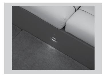
Courtesy lights are installed at several locations in the interior of the boat. The courtesy light switch is located on the instrument panel and is marked "COURT".
