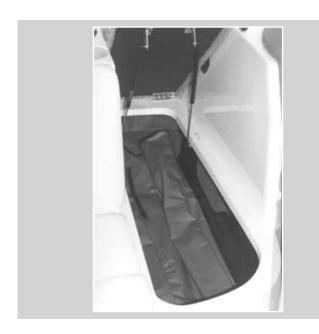
Care should be taken that the ballast bags are situated properly with the fill hose on top and drain hose on bottom and that all fittings are installed securely. The bags should not be twisted and the bags should be free to expand and drain completely. Care should be taken to prevent sharp objects from coming in contact with the bags. Cuts and punctures to the bags are not warrantable.
