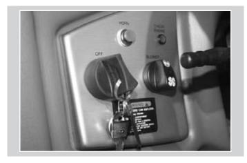
Located on the port side of the dashboard, the ignition switch has four positions. In the vertical position, the ignition is "OFF".
