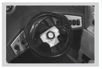
Tilt steering may be adjusted up or down in five different locking positions. To adjust, depress the tilt lever located beneath the bezel and move the steering wheel to the desired position. Release the lever to lock the wheel into place.
