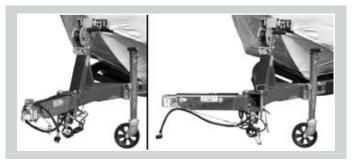
With the swing tongue, you can shorten the trailer length for storage by pulling the pin and swinging the tongue away to the side.
