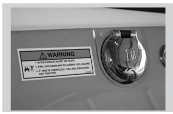
NOTE: The gas cap is sealed by a rubber O-ring. Ensure the cap is clicked shut to properly seal.
