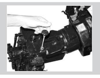
Pull the V-Drive Oil Level dipstick to check the fluid level. If the level is low, add fluid to the correct mark on the dip stick. Use SAE 15W-40 motor oil.
