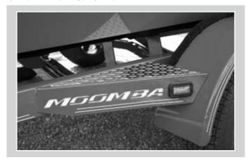
The optional laser cut steps are backlit so they illuminate when the trailer's running lights are illuminated.
