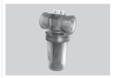
The optional ballast system also includes an in-line water strainer before the manifold. This strainer will keep debris out of the solenoid valve and should prevent the valve from getting clogged up and forced open. The strainer cover should be removed periodically and the filter screen cleaned to prevent debris buildup on the mesh screen. Be careful when removing the cover not to lose the O-ring used to seal the cover. Also, the strainer should be removed and drained during winterization.
