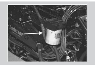
In the V-drive engine configuration the remote oil filter is mounted in a convenient spot in the engine compartment.
