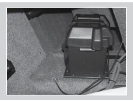
The battery box is mounted on the inside of the observer's seat storage compartment.
