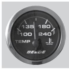
The temperature gauge indicates the engine coolant temperature while the coolant is circulating inside the engine. Engine operating temperatures will vary depending on the weather conditions and engine load. Normal operating temp range is between 160 degrees and 180 degrees.
