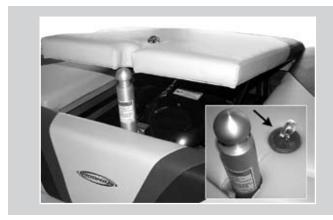
To access the engine compartment, turn latch and pull to raise the center sun deck lid. When the ski lockers and engine compartment lids are closed, the upholstered lids double as a cushioned sun deck.
