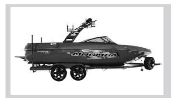
The trailer supplied with your Moomba model was designed especially for the boat with your convenience in mind. Please be sure that you have an appropriate tow vehicle before attempting to trailer your boat. Your vehicle must be capable of towing 3,500 — 6,000 lbs., depending on the model.
