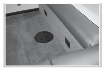
On all V-Drive models, the fuel pump is located beneath the floor in front of the rear seat. The pump may be accessed by twisting and removing the access cover.
