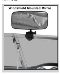
The rear view mirror is installed as a standard item. The mirror is adjustable so that it may be set for each driver.
