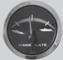
This switch controls the optional wakeplate. The gauge indicates the position of the wakeplate.
