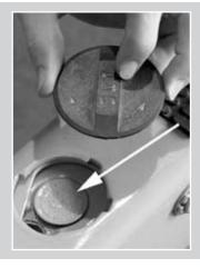
To check brake fluid, twist black cap and remove. Pry rubber plug out of reservoir. Follow instructions printed on plug. Use DOT 3 Brake Fluid.
