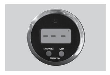
If the display indicates three horizontal bars as shown, the depth sounder indicates an out of range, inaccurate or incomplete data condition.
