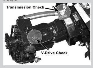
Transmission fluid level should be checked regularly (such as every ten engine hours) and fluid added if necessary.
