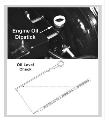
If the oil pressure indication is too high or too low, stop the engine immediately and check the oil level on the dipstick.
