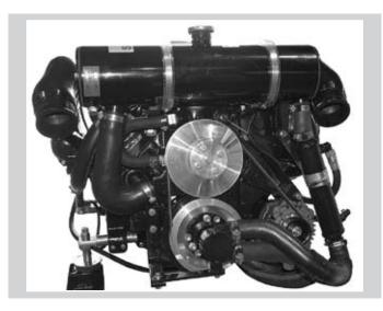
The optional fresh water cooling system has a heat exchanger which allows the engine to have an antifreeze mixture which circulates in the engine. For more information, see your engine owner's manual.
