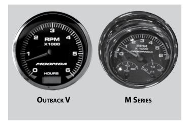
The tachometer registers the operating speed of the motor's shaft output and may be used as an alternative to speedometer if weight and water conditions permit.
