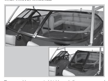
The moveable center windshield panel allows access to and from the bow area on some models. To open, turn safety latches to vertical and push. Carefully lay the hinged windshield panel back against the fixed side panel.
