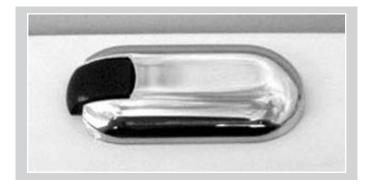
The pole light receptacle is located on the port side deck near the stern. To install the pole light, open the cover completely and with the plug correctly aligned, slide it into the socket until the electrical contacts are firmly in place.
