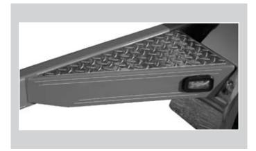
The optional aluminum step plate gives the trailer a durable long-lasting, nonskid surface on the trailer steps.
