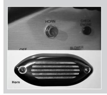
The Horn Switch is located on the switch panel to the left of the steering wheel.
